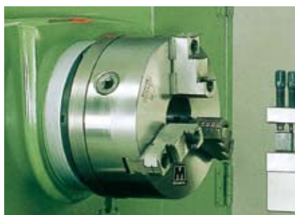
1. 強力三爪夾頭(SK) 3-Jaws strong scroll chuck
