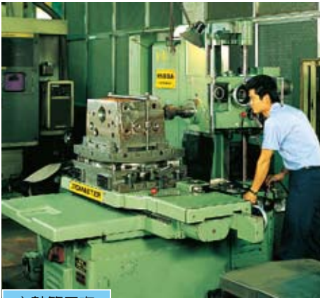
2nd finished machining for Headstock
